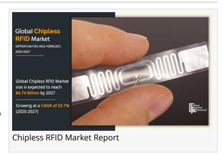
chipless RFID system provide identification data & monitor several physical parameters of tagged items without having an active sensor in the circuitry.
