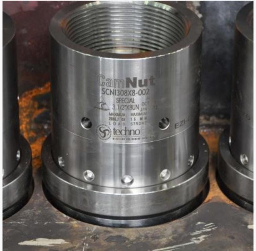
Normally, a bolt tensioning tool pulls on the bolt threads protruding above the regular hex nut, which is then screwed down to retain the loads induced by hydraulic operation of the tool. With no available thread, the CamNut (pictured) performs as the con
