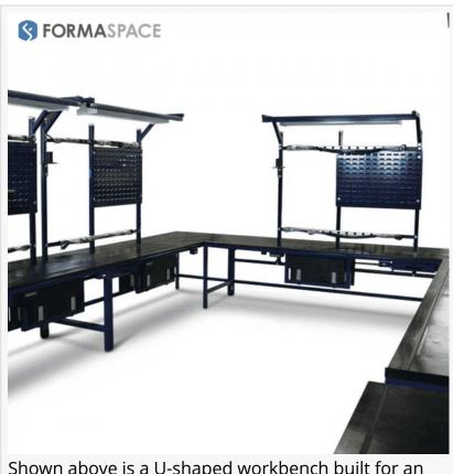
Shown above is a U-shaped workbench built for an electronics manufacturing company, which features our proprietary ESD protective surface that keeps sensitive electronic components safe from static electric shocks.
