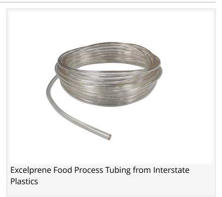
Excelon Excelprene food process tubing, a Tygon® A-60-F equivalent, is made from a thermoplastic elastomer (TPE). Formulated specifically to withstand the extreme temperatures that arise during many food, dairy, and cosmetic processing applications, it can operate from -75°F to 275°F without issue.
