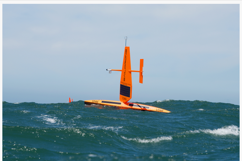
A 23-foot Sailable Explorer sails in waves during an ocean data collection mission in the Pacific Ocean.
