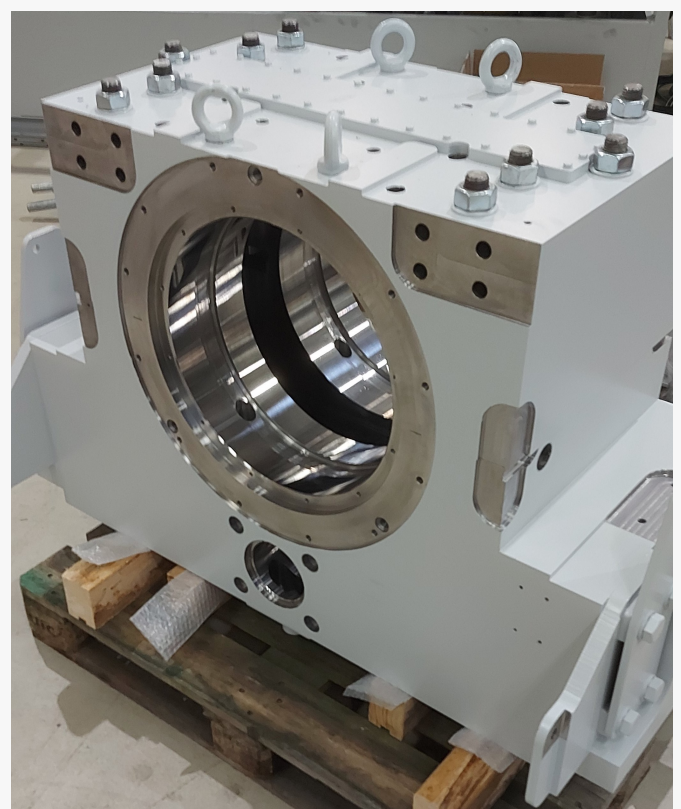
R&D Test Systems' test rig and its outer bearing support structure developed for the Rolls-Royce UltraFan
