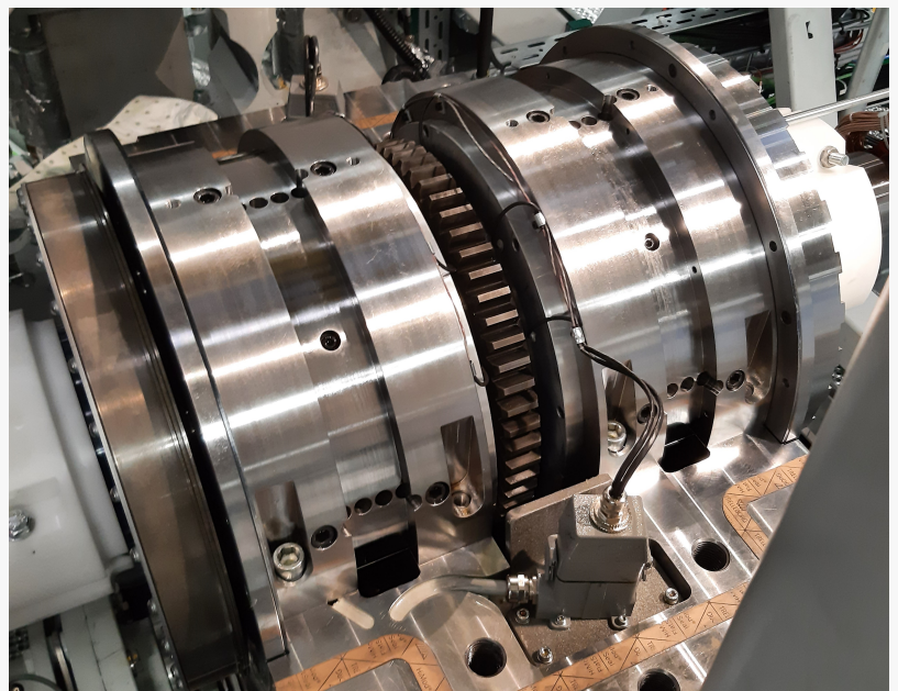
Core of the bearing test bench developed by R&D Test Systems for Rolls-Royce UltraFan project
