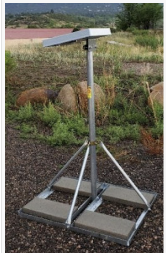
The next wave of Hailios sensors is ready to be deployed across the world to provide ground-level data regarding hail damage, frequency, and size.
