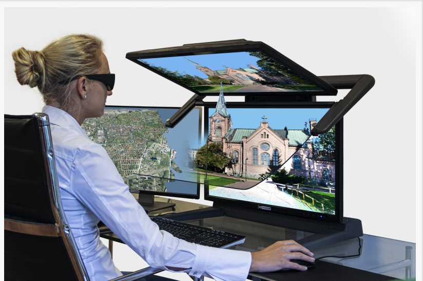
Passive beam splitter technology for demanding GIS workflows: The 3D PluraView monitor from Schneider Digital.
