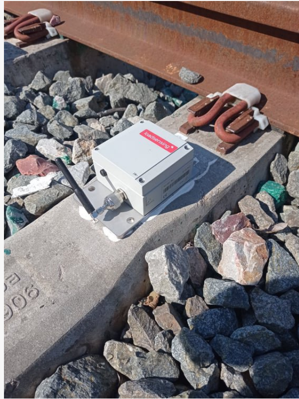
Tiltmeter on rail track
