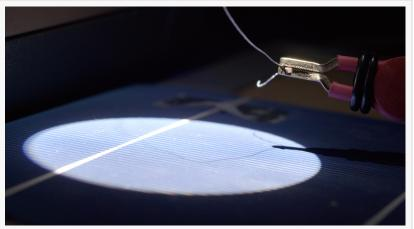
IntriEnergy's novel anti-reflective coating is based on a diamond-like carbon structure that utilizes a simple one-step application, achieving near-zero reflectivity (99%) over the entire solar spectrum.
