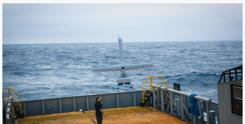
A Shield AI engineer watches as a V-BAT unmanned aircraft is launched from the deck of a small vessel during sea trials conducted on behalf of the Canadian Coast Guard.
