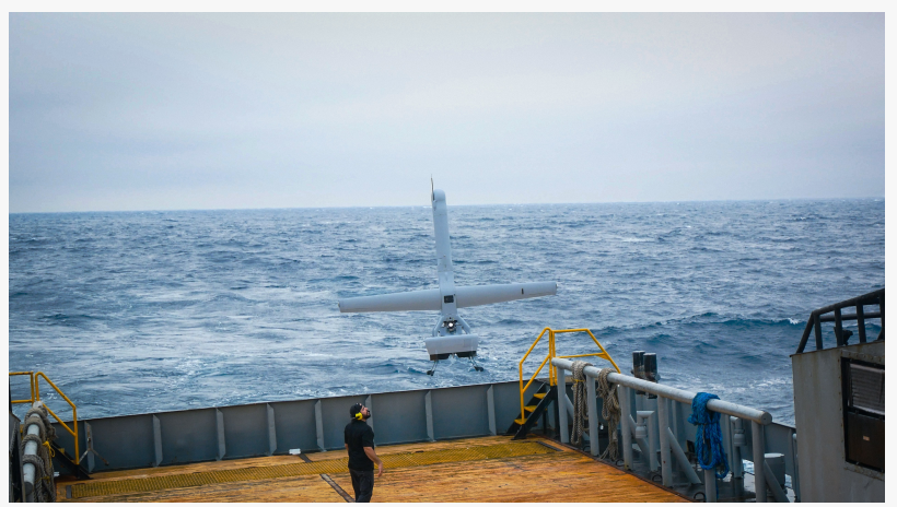
A Shield AI engineer watches as a V-BAT unmanned aircraft is launched from the deck of a small vessel during sea trials conducted on behalf of the Canadian Coast Guard.
