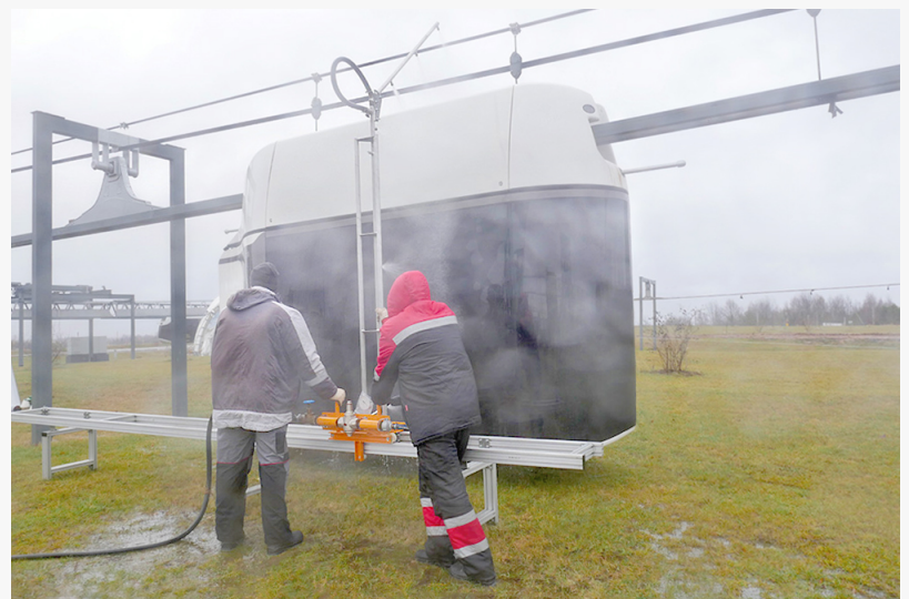
The testers simulated a tropical downpour using a special watering machine.
