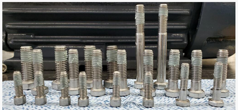
Environmentally-friendly LOX-8 Paste is used on CRYO-MACH's threaded connections
