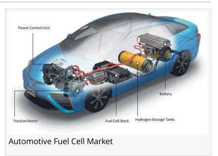
economical and attractive option for mobility with zero emissions. A fuel cell-electric vehicle is an electrically driven vehicle in which electricity is generated by a fuel cell using hydrogen as an energy source. Alternatively, this energy can be temporarily stored by the traction battery. Additionally, fuel cells have a higher efficiency than diesel or gas engines. Moreover, most fuel cells operate with a low noise level as compared to internal combustion engine.
