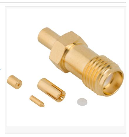
SMA connectors are lightweight and compact and offer reliable RF performance up to 6 GHz. Their high-strength design and threaded coupling mechanism combat vibration which aids in providing secure mating. These SMA jacks are constructed with gold-plated, brass bodies with gold-plated, beryllium copper contacts. They utilize a larger back end to increase the compatibility options of other connectors that can be paired with them.
