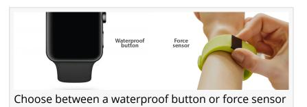
Force sensing, however, happens when the user squeezes the housing of the application to produce the desired action – such as unlocking the screen. Force sensing is a popular user interface for wearable applications, as it is not prone to false activations. It is also a more robust and reliable interface than capacitive sensing in applications that tend to get wet or damp, or where the user is wearing gloves, such as in wearables that are used in more active lifestyles.
