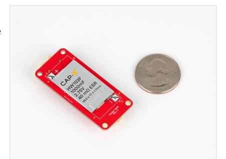
Offering power buffering in Adafruit Feather form factor designed for open-source maker community, MCCI Model 4906 Supercap FeatherWing LoRa Module features 1F CAP-XX supercap to store energy and deliver burst power for wireless transmissions in IoT devices
