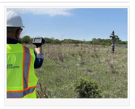
detection devices for use primarily in its Appalachia operating area, which will complement the company's demonstrated operational focus on environmental stewardship. Portable methane emissions detection devices will empower Diversified's personnel to identify and remediate emissions otherwise undetectable using traditional techniques.
