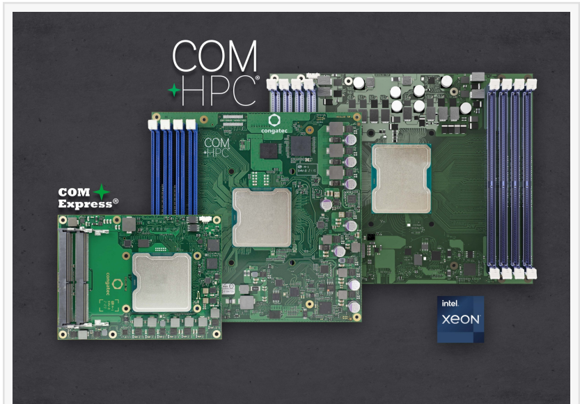
congatec's Intel Xeon D-1700 and D-2700 processor based Server-on-Modules in COM HPC Server Size E, Size D and COM Express Type 7 form factor (from right to left)
