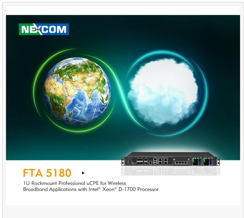
In response to the growing demand for wireless, flexible, and space-saving edge appliances, NEXCOM developed FTA 5180 which perfectly covers all these key areas while maintaining excellent performance. Powered by Intel® Xeon® D-1700 processor, FTA 5180 is equipped with ten high-bandwidth Ethernet ports to deliver high throughput and handles cryptography acceleration with ease via with embedded Intel® QAT.
