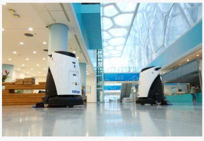
Powered by AI technologies, Scrubber 50 has a high level of environmental perception and obstacle avoidance. The subway Line 11 has had a large passenger flow during the Winter Olympics. The robots could work competently in such dynamic environments, dexterously avoiding the passengers while cleaning.
