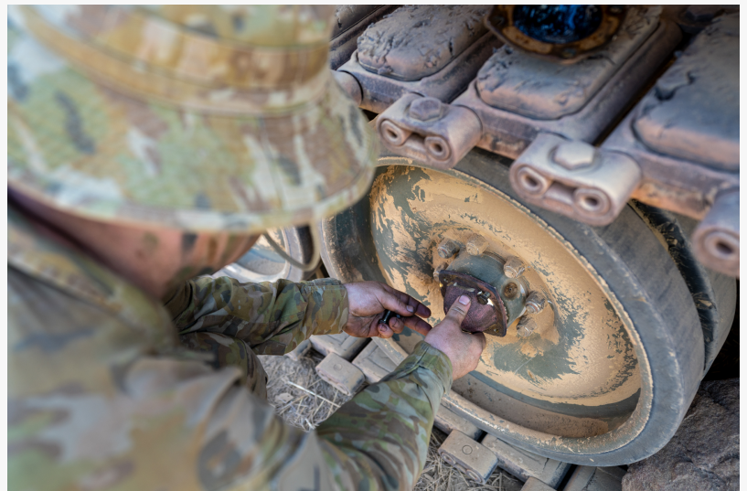
Bradshaw Wheel Bearing Installed on M113 vehicle by Australian Army Soldier
