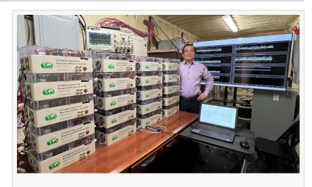
to solar panels in the field and seven of the inverters are connected to batteries so two of the inverters are connected to both solar panels and batteries. The inverters can black-start by itself, synchronize with each other, connect together to form a grid, regulate the voltage and the
