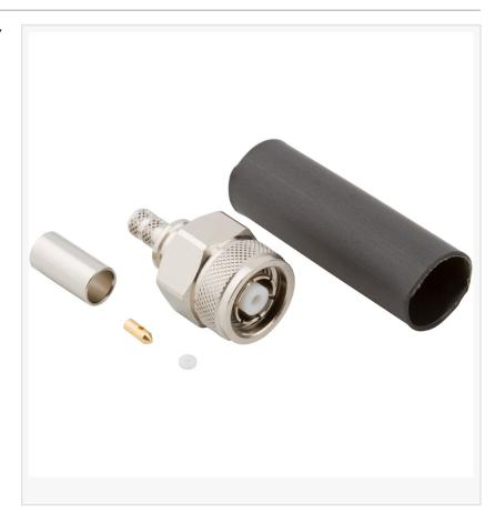
The new RP-TNC connector offers reliable electrical performance up to 6 GHz while providing versatility in mating options with its secure, familiar threaded coupling mechanism. This ruggedized solution is constructed with a brass body and bullet contact, and PTFE insulator components. The interface contact is made from gold-plated, beryllium copper to ensure proper mating to standard RP-TNC jack connectors.
