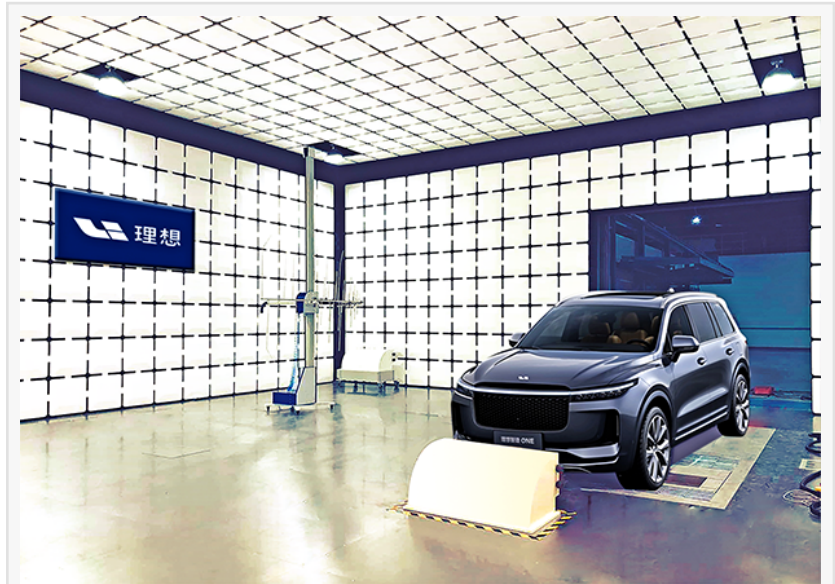
Example of TOYO's EMC Test System for Vehicles in Use
