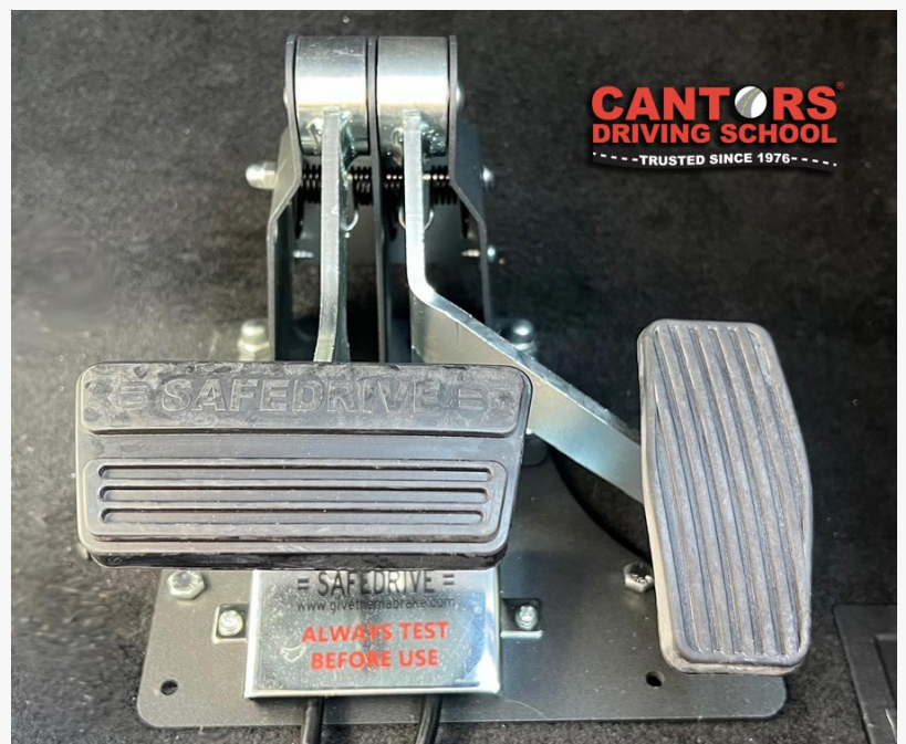
Instructor Dual Brake and Gas Pedals in Cantor's Driving School FL Driver Training Car
