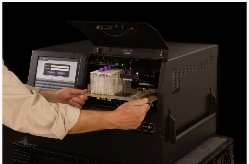
An F7-Chip is being loaded into an ANDE 6C instrument.
