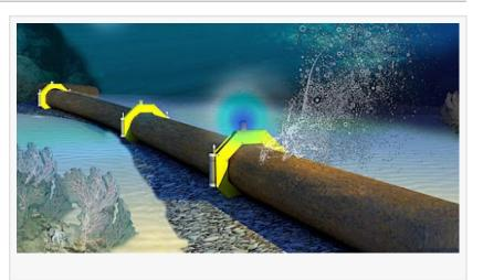
detecting the leak location in a pipeline. Leakage is identified using acoustic and non-acoustic devices. A water pipeline leak detection system includes various sensors and data collectors that are placed within the pipeline network and transmit data to the network management center, which helps in identifying the leakage area. These detection systems assist in reducing the cost of water supply and find widespread applications across the commercial, industrial, and residential sectors.
