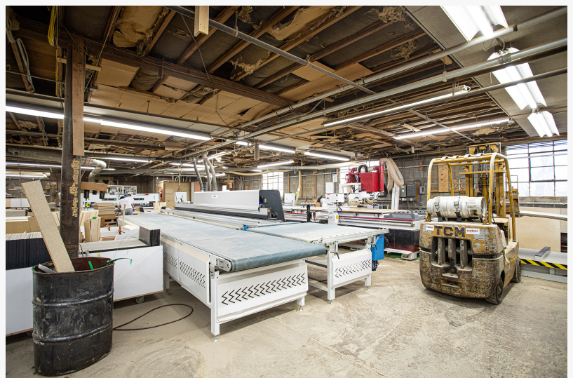
An integrated return on CNC Factory edgebander eliminates labor on re-feeding each edge of the panel.
