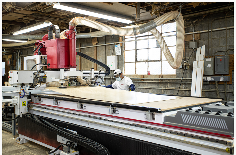
An automated assist speeds panel processing through Cober Cabinets' router from CNC Factory's Python XPR
