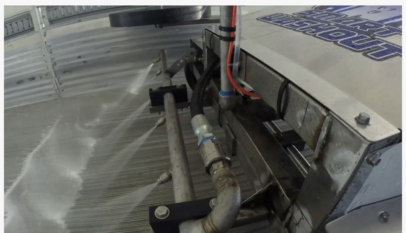
internal trailer wash system for semi truck
