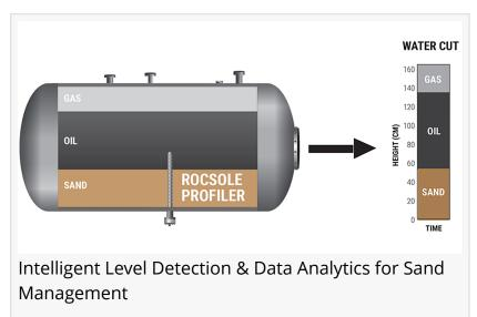
reduced production rate. ROCSOLE utilizes leading-edge tomographic technology, its Separator Profiler is a real-time non-radioactive monitoring solution that physically sees and measures separator's emulsion layer, improving separation efficiency by optimizing residence time and
