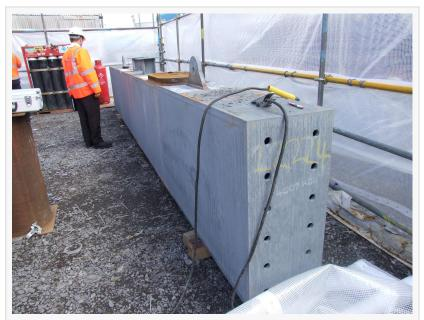
The example shown refers to a very large steel section, too large to fit in regular galvanising tank, galvanised on site.
