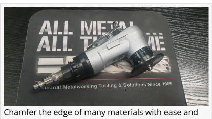
speed with this chamfering tool.
