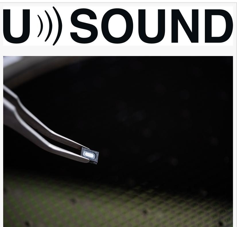
USound MEMS loudspeakers are available without ferromagnetic materials and are fully compliant to manufacture MRI-compatible headphones.
