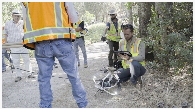
Caged LIDAR system, for lowering into confined space
