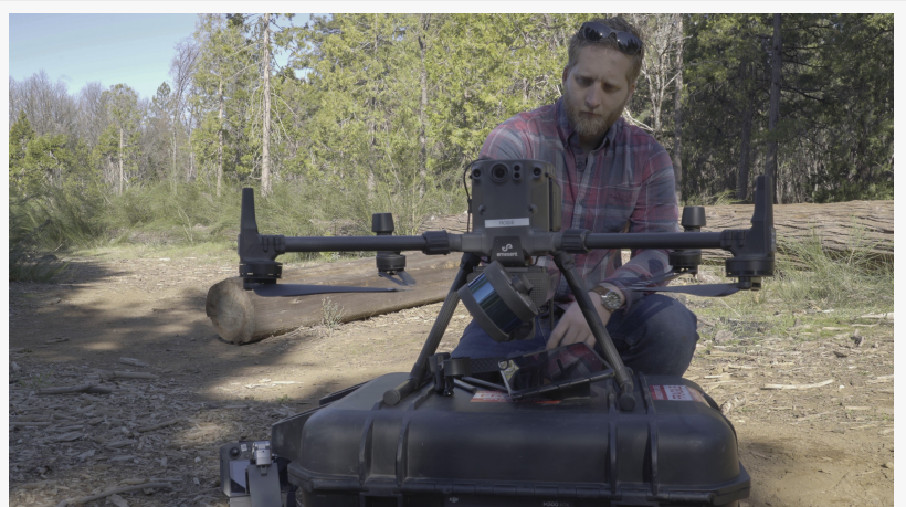
Fully Autonomous lidar system, mounted on a drone
