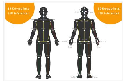
VisionPose detects up to 30 keypoints of the human body in 2D, and 17 keypoints in 3D.
