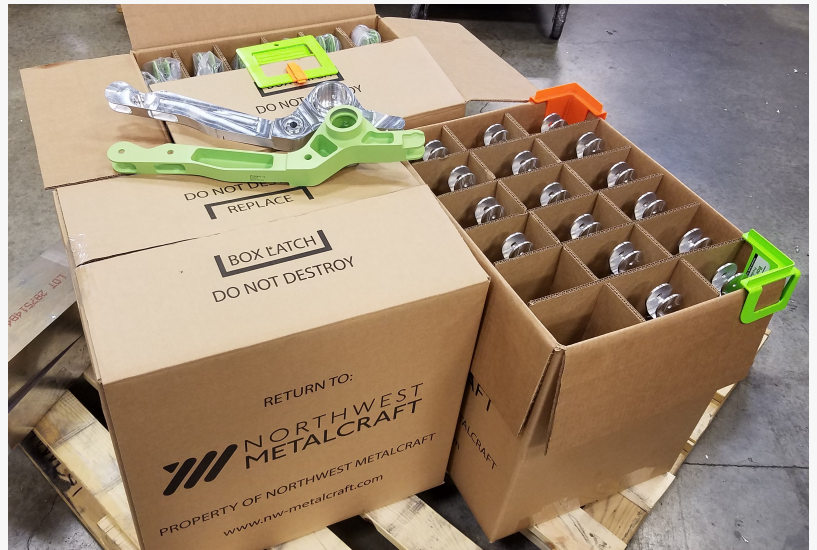
Custom designed reusable box to transport aircraft parts
