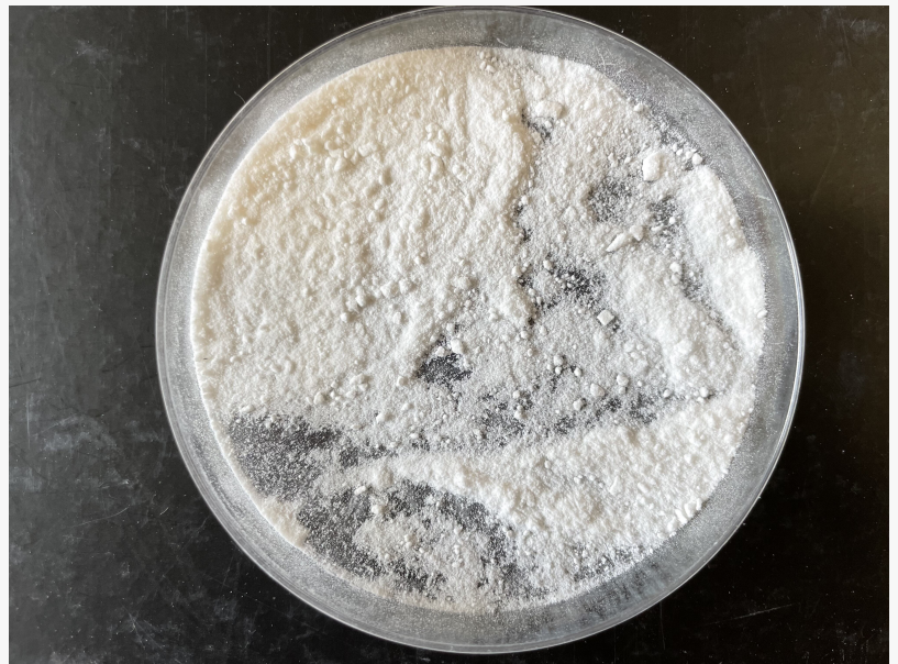
Lithium carbonate produced using Ekosolve Direct Lithium Extraction process from high magnesium brine
