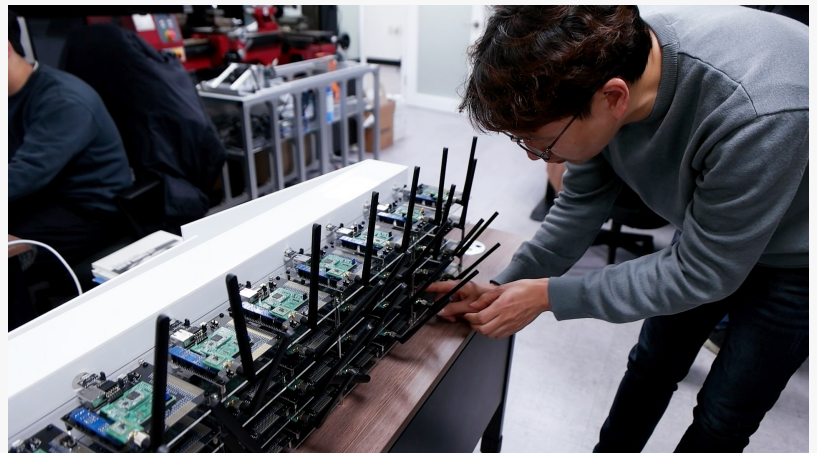
DongKeun Kang, Head of Research at SDT, tests the Wi-SUN Mesh Network
