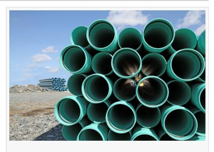
construction and electrification purposes. These pipes are resistant to chemicals and high fluid pressure which makes them fit for distribution of potable <u>water</u>. They are used for renovation and often substitute traditional materials like wood and metals. PVC pipes are not only durable and light in weight but are also cost-effective and easy to install. Their high degree of inertness and resistance to corrosion makes them an ideal choice for use in earthquake-prone areas.
