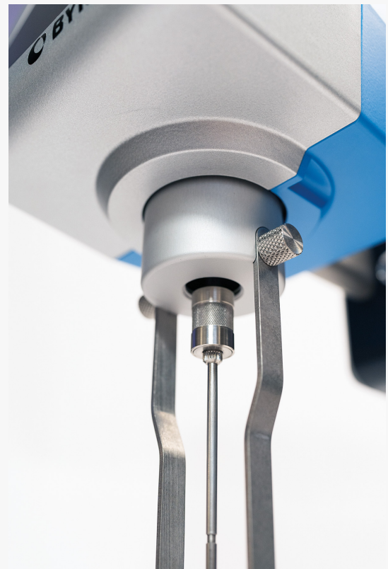
Easy byko-visc snap-on spindle attachment allows you to quickly switch out spindles with no effort
