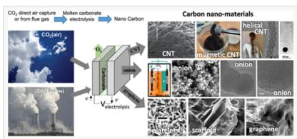
High-yield electrolytic synthesis of carbon nanomaterials produced from CO2, either directly from the air (Direct Air Capture) or from smokestack CO2, in molten carbonate.
