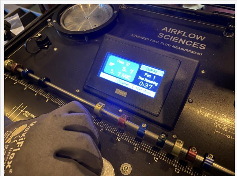
The new PLC interface on the ACFM V3 provides unparalleled reliability, even in harsh testing conditions and the integrated weigh scale reduces the need for peripheral equipment, resulting in an even more compact and portable test setup.
