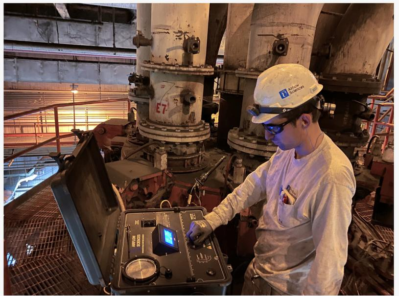
The ACFM is equipped to perform clean air tests, dirty air tests, and isokinetic sampling. The complete system also ensures compliance with international test standards such as ISO 9931 and U.S. standards such as ASME PTC 4.2. Power plants with specific testing requirements can customize the ACFM to meet their operational needs.
