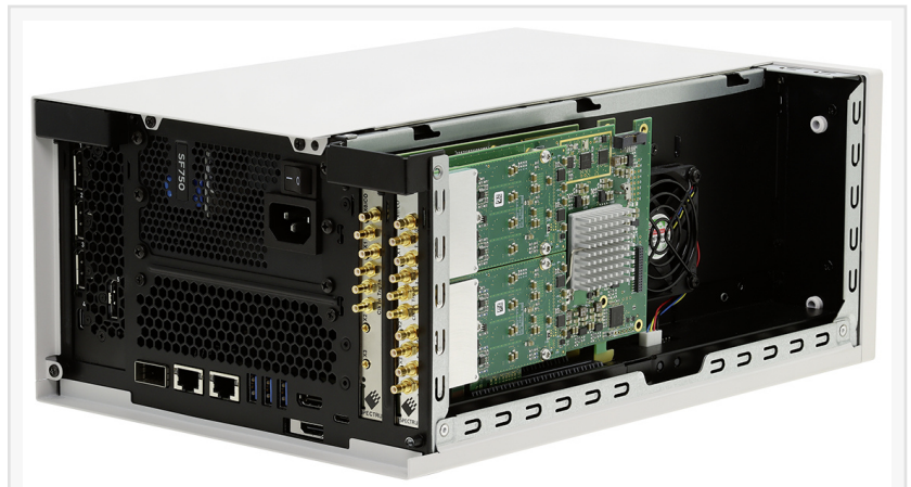
Pic 2: NVIDIA Clara equipped with two SPECTRUM cards: 4 channel signal generation plus 8 channel signal acquisition with 125 MS/s
