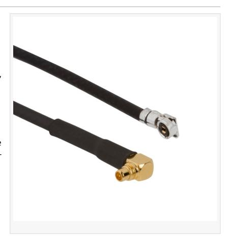
MMCX connectors are manufactured from brass with gold plating while the ultraminiature AMC4 features a silver-plated phosphor bronze body. The assembly offers secure and reliable mating with the quick connect/disconnect snap\(\text{D}\) on coupling mechanism. The MMCX to AMC4 assemblies offer reliable electric performance up to 6 GHz.
