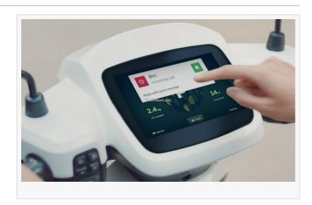
automobile telematics products especially for the India and Southeast Asia markets. The products include in-vehicle-infotainment system (IVI) and Telematics Control Unit (TCU), for two and three wheelers – also called electronic scooters or Ebikes . All of these products are based on technologies in Qualcomm chipsets.
