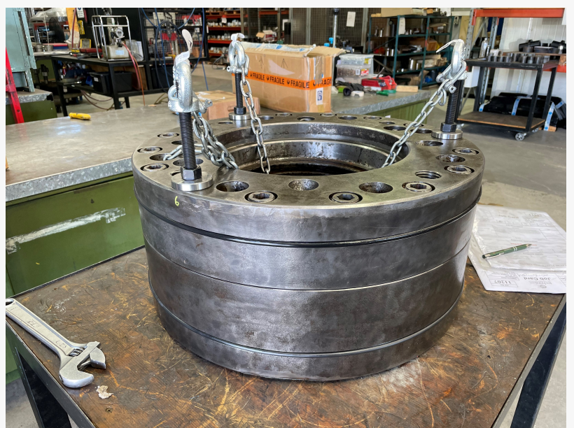
A large diameter EziTite Head Nut at Technofast's warehouse in Queensland, as it is prepared for dispatch to a mining customer
