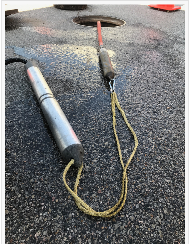
Ruggedized probe able to automatically identify and measure defects in Gallons of Minutes or Liters per Seconds of Each Leak Precise to 0.4" or 1cm.
