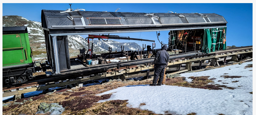
Built in-house Rerailing car
