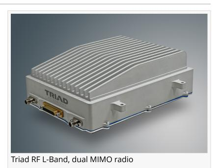
The THPR1039 is a 10W (5W per channel), <u>L-Band, dual MIMO radio</u> that is used for long-distance UAS Video and C2 links, which achieves RF link ranges in excess of 50km when used in both the ground and air radio segments. This unit is an expansion of Triad's High-Power Radio System (THPR) product line. It combines a DTC Solo8 MIMO radio, high-power amplification, and custom
